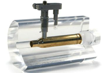
Figure 3: Barrel Pressure Sensor
